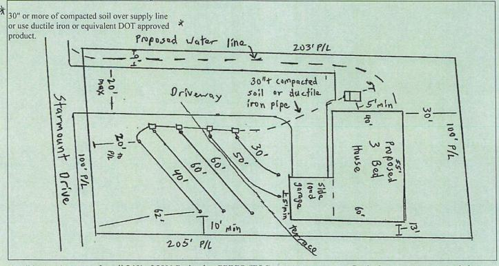
Condition(s) of Issuance: Install 240' of 50% Reduction PPBPS (T&J) system on contour. Grade down terraces as needed to improve surface water flow. Maintain 10' from any property line, 10' from any water line, and 5' from any building foundation. Install according to all NC Rules and Regulations. Install according to T&J installation manual.
